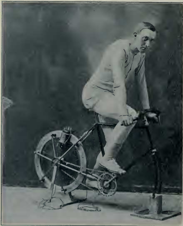
FIG. 3. Bicycle ergometer for studying problems relating to muscular work.
